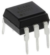
This Triac Optocoupler looks like an IC. (Image source)
